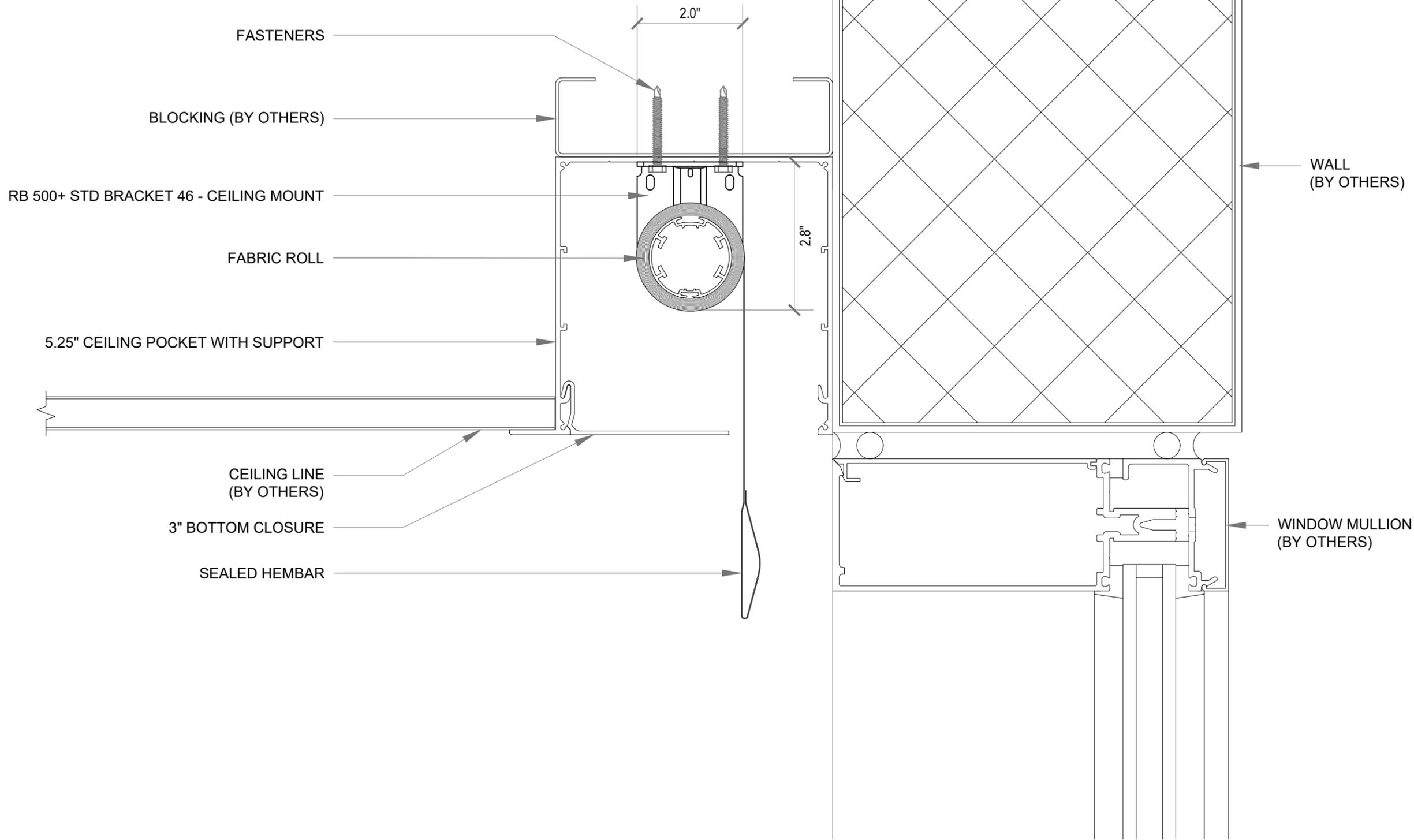
**01 RB 500+ STANDARD DUTY BRACKET 46 - SECTION DETAIL**
